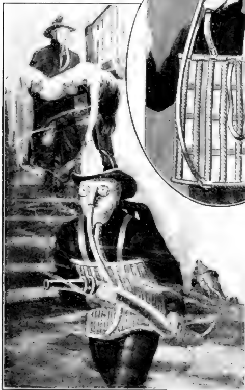
The suit is provided with numerous tubes through which air passes to the wearer
